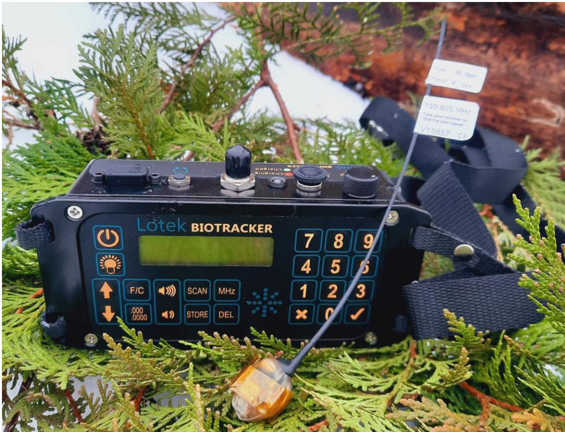
Figure 6: VHF receiver and 25g training transmitter. The transmitter for the deer weighs 7 grams.
